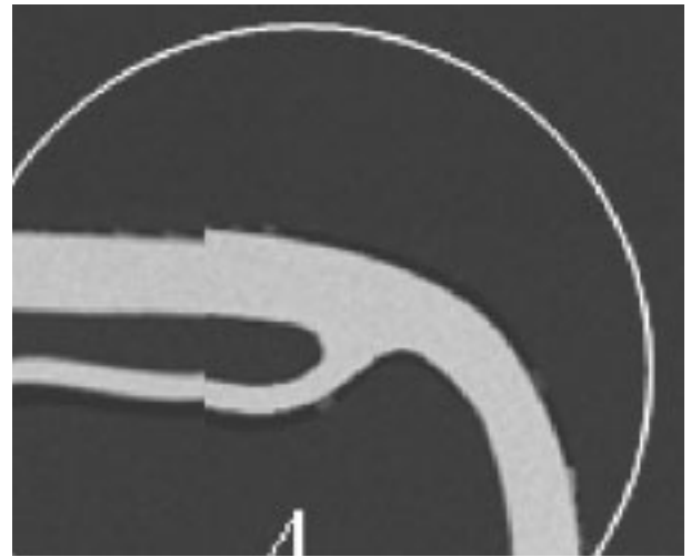
b) Joints made of 304LN stainless steel and brazed with MBF-51 foil
